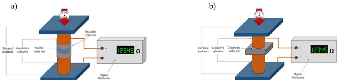
Figure 1: Sketch of Measurement set-up for conductivity study of a) carbon fillers and b) composite
