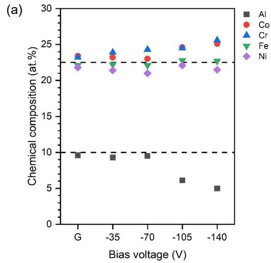
Fig. 1: (a) Chemical composition of HiPIMS-deposited AlCoCrFeNi HEA thin films as a function of the substrate bias voltage.
