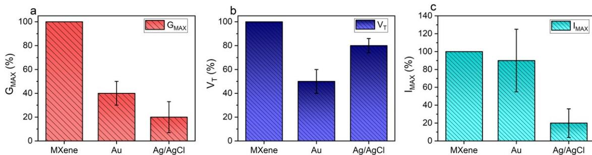
Figure 1. Percentage variation of the transconductance (a), threshold voltage (b) and maximum current (c) of the OECT gated with MXene, Au and Ag/AgCl. All the values were normalized to the MXene gate.
