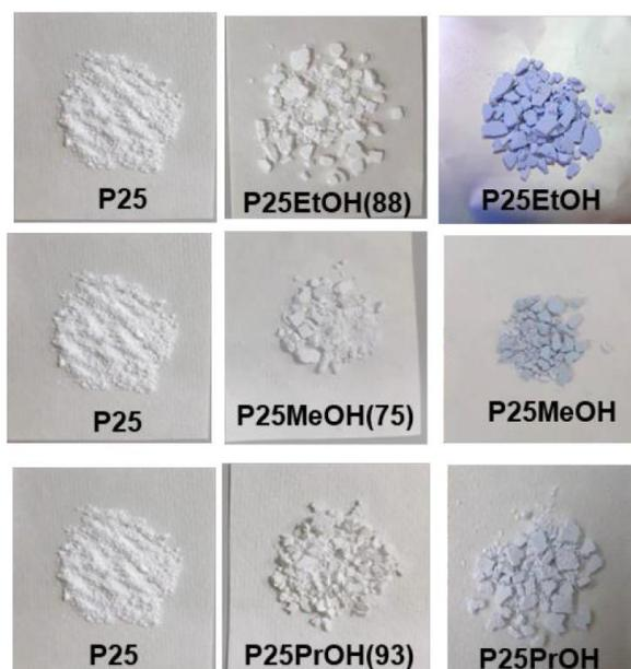
**Figure 1:** Image P25 powder before (left column) and immediately after (center and right columns) a 24 hours refluxing treatment in three different alcohols (Top row: ethanol; center row: methanol; bottom row: 2-propanol) and at two different oil bath temperatures: T<sub>1</sub>=T<sub>b</sub>+10°C (center column) and T<sub>2</sub>= 120°C. Here T<sub>b</sub> indicates the boiling temperature of the different alcohols.
