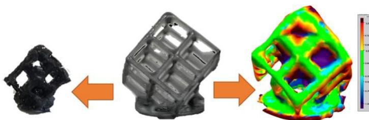
Figure 1. MXene/composite 3D printed structure. On the left, there is a carbonized treated sample. On the right, 3D scanned heatmap.
