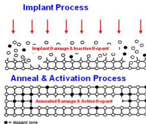
Figure 1. Schematic of the silicon implantation and successive annealing (reprinted from intechopen.com).
